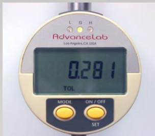
Gauge showing "Go" for Good reading within range
