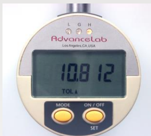
Gauge showing "H" for reading too High
