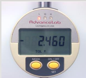
Gauge showing "L" for reading too Low
